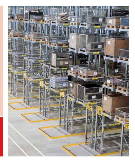
Narrow Aisle Pallet Racking is your ultimate space-saving option if your warehousing or storage floor space is limited. It gives your teams maximum storage capacity, and allows for quick orderpicking and fast accessibility to every pallet.
