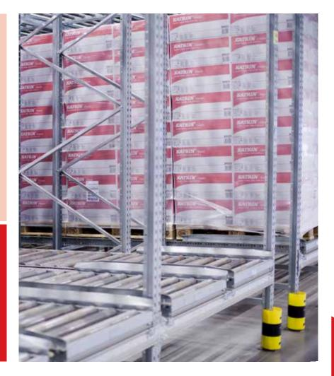
Pallet Flow Racking, or 'Pallet Live Storage' is ideal if you operate a First-in, First-out (FIFO) goods storage setup. With this system you can use up to 60% less space than if you were to use conventional pallet racking.
