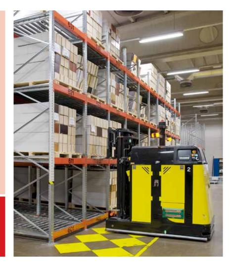
Push-back Rollers – a dynamic storage solution based on the CR18 Pallet Racking System and including wheel/roller conveyors. Ideal if you're storing bulk goods on pallets according to the Lastin, First-out (LIFO) principle.
