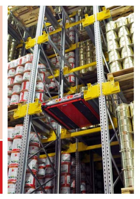
The Pallet Shuttle system is a semi-automated, high-density storage solution for the handling of goods inside channels similar to a drive-in or pallet-flow setup.
