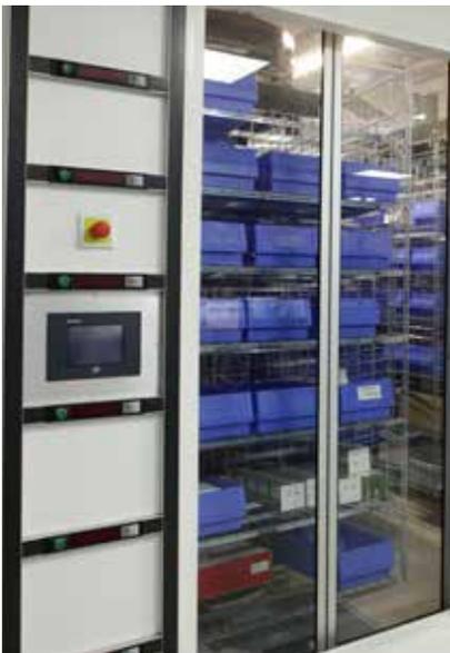
The Horizontal Carousel (HOCA) Automated Storage Machine is a computer-controlled storage and transfer solution that significantly improves the efficiency of product storage and picking.
